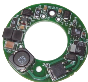
Single LED Driver Module
