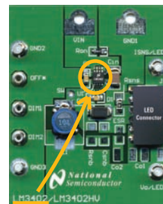
LM3402/02HV evaluation board with female 6-pin SIP connector and two standard 94 mil turret connectors for easy connection to LED array
