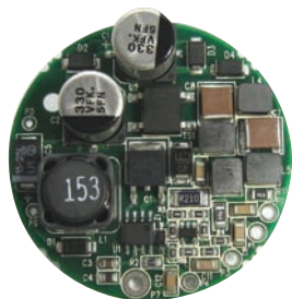
Multiple LED Driver Module
