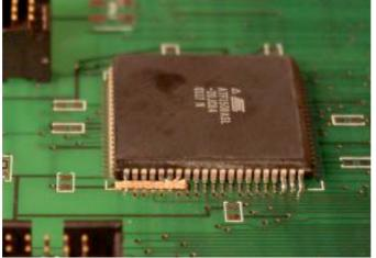
3. Take your soldering iron and heat the solder wick, which will heat the solder on the other side which will absorb into the solder wick
