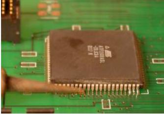
4. When the solder goes into the solder wick (with the small wick used here it should only take a few seconds) remove both the solder wick and the soldering iron. Likely that area of solder wick will now be full of solder and useless, so clip it off (unless you already did that). Note that this very fine solder wick used here fills up very fast, so you might also want a wider roll as well if you need to remove a fair amount of solder.
