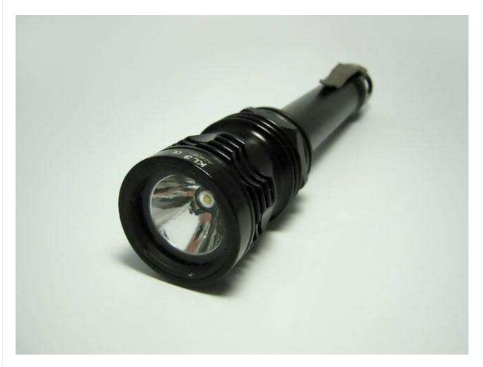
KL3 with a modified Pelican M6 reflector. Mr "fixer", who is a machinist of <u>ROF-1</u>, kindly made a turned down reflector and some spacers for me. I changed resistors on the stock KL3 circuit to deliver 1 amp to LED and replaced the LED with Luxeon III high dome.
