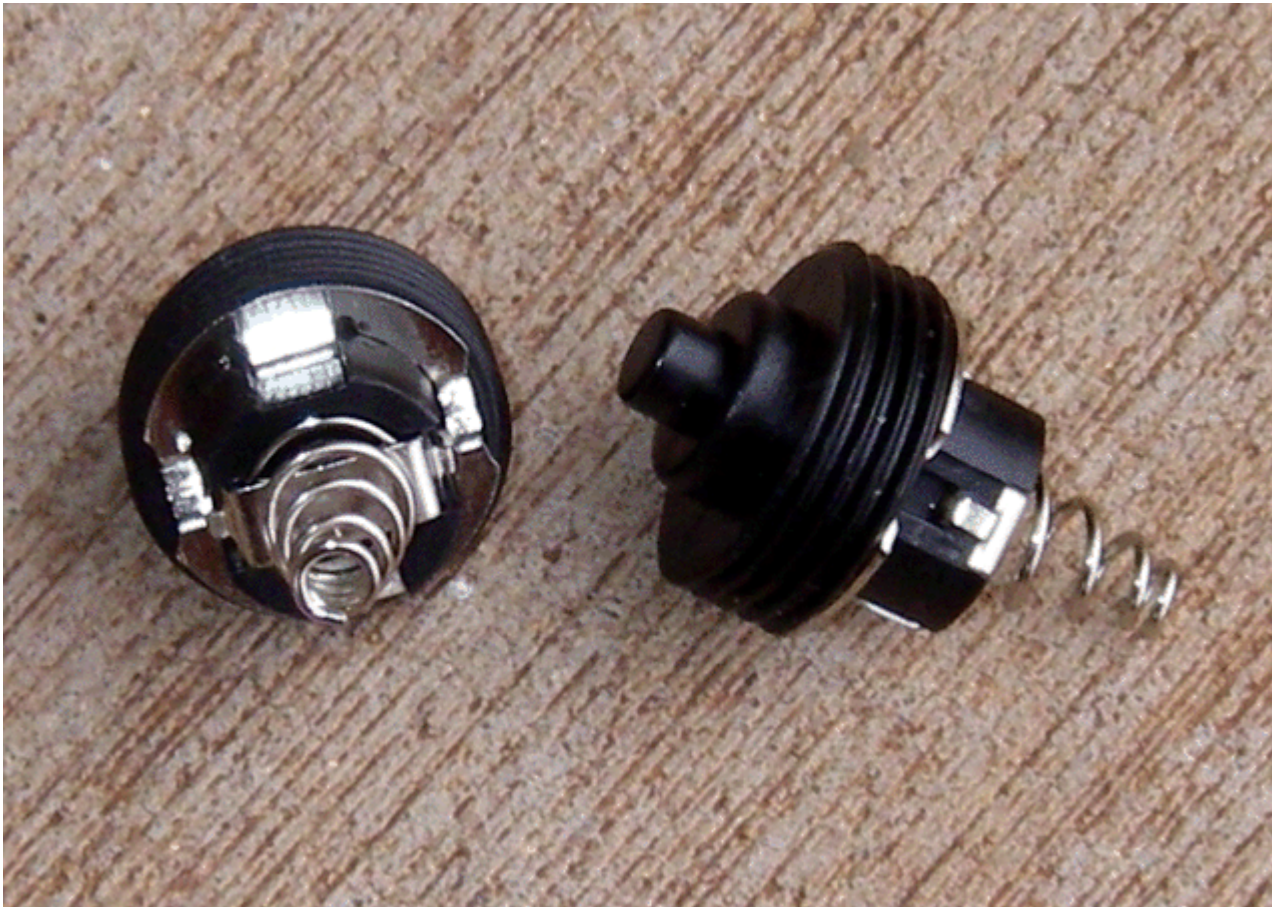
McClicky switch module ... a universal clicky switch module that will fit the new McTC Tailcap (see below) or any Aleph Tailcap ... or any other host you design for it. It offers momentary and constant mode and is not a reverse clicky.
