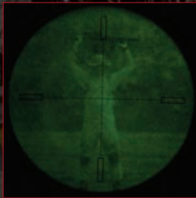
Subject at 70 yards illuminated by ambient light. Photo taken through AN-PVS26 paired with a Nightforce™ optic.
