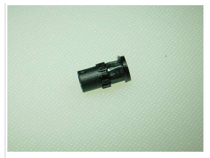
Pull out the two switch connectors, cut the back one down even with the switch so it will no longer make contact with the positive battery spring slug and solder a small wire (24 AWG or smaller) to the inside of it and then do the same to the front connector, it doesn't need to be cut down.
