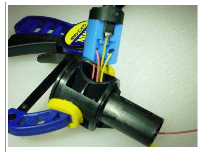
Snip off the excess ground strap, solder the negative power supply wire to it and feed it up through the bulb post.
