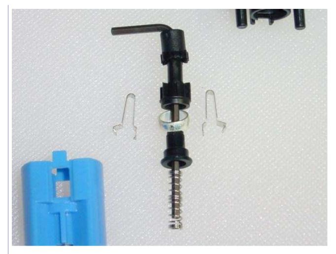
Find the two pieces in the top half of the switch one part meets the rubber boot cover, the part below it is what needs to be modified by cutting the outside ribs off so the switch no longer clicks. I use a hobby knife "razor blade" to trim them off. This will allow the switch to cycle up and down in the momentary mode with out clicking, locking into the on/off mode.
