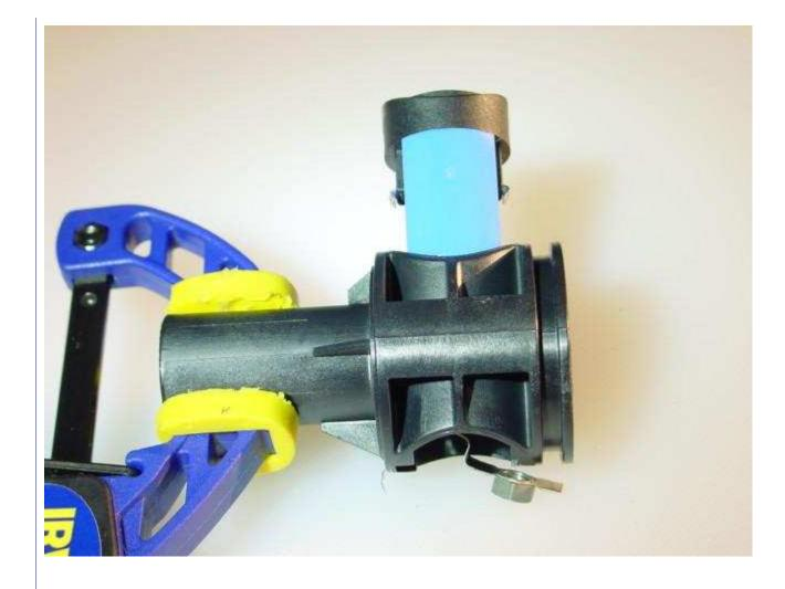
Carefully separate the switch core by pulling on the black top half and the blue bottom part.
