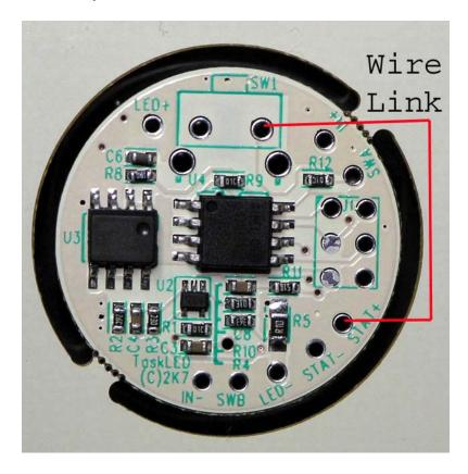
If at a later time you want to make the slave act like a master again, all that is required is to remove the wire link. The bFlex will then revert back to running as a master.
