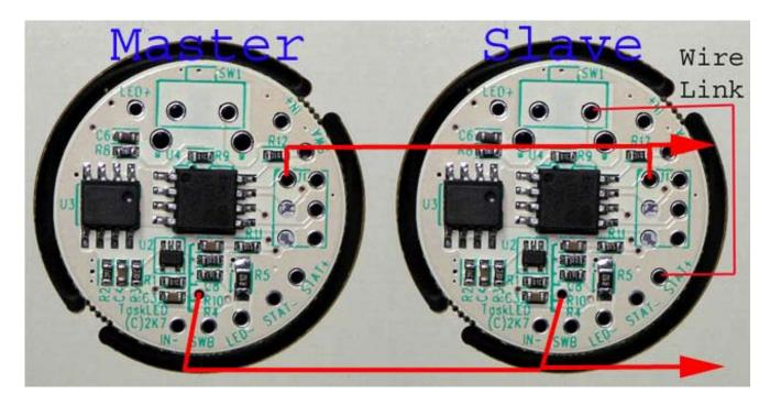
The IN+ of both master and slaves should be wired to the battery+. The IN- of both master and slaves should be wired to the battery-.
