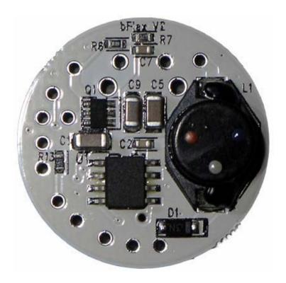
When soldering wires to the through holes/pads on the PCB, be careful to not short or accidentally desolder components near where you are soldering. Use a quality solder with non-corrosive, non-conductive (no clean) flux.
