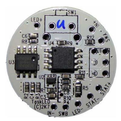
The picture shows the connections to bFlex-V2B. The user provides DC power to the bFlex (via battery, DC wallwart, vehicle/boat/RV 12V. bFlex is reverse polarity protected with a low drop out FET (less than 50mV voltage drop across the FET).
