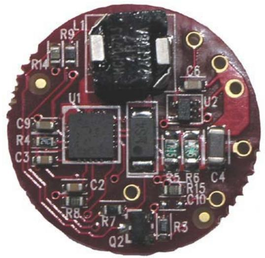
When soldering wires to the through holes/pads on the PCB, be careful to not short or accidentally desolder components near where you are soldering. The following table shows the supported configurations of maxFlex3.
