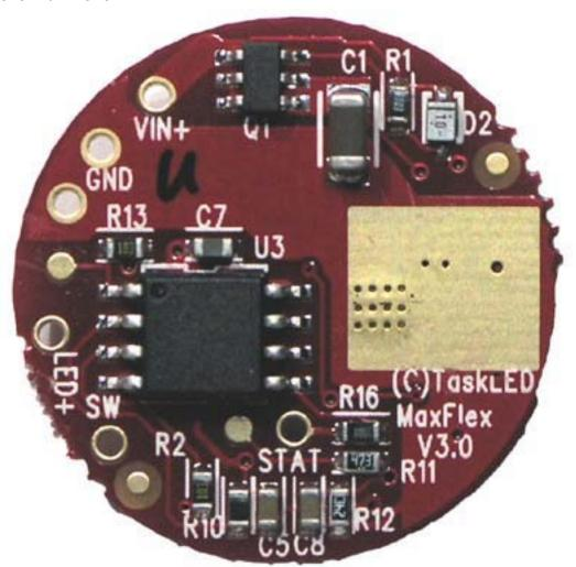
The picture shows the connections to maxFlex3. The user provides DC power to the maxFlex3 (via battery, DC wallwart etc.
