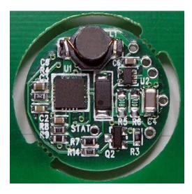
**Note**, MaxFlex is a Boost regulator (step up), so input voltage must be less than the output voltage to ensure MaxFlex remains in regulation. If the input voltage exceeds the output voltage (at the dialed in drive current), MaxFlex will no longer regulate and the input voltage will go through the series inductor and schottky diode directly to the load. This will cause the output current to a LED to rise rapidly since LEDs have a very steep Current vs Voltage curve (Vf).
