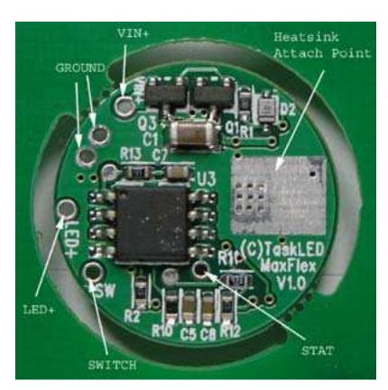
The picture shows the connections to the MaxFlex. The user needs to provide DC power to the MaxFlex (e.g. battery, DC wallwart etc).
