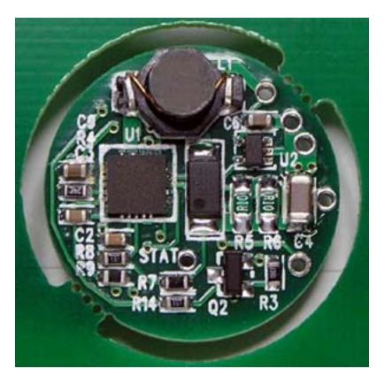
As shipped, the MaxFlex is configured for nominal 350mA drive. The user may reconfigure the MaxFlex drive level as described later in this document.
