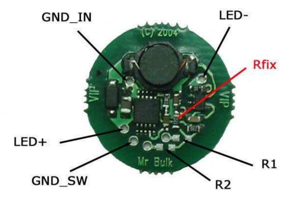
The VIP driver is a boost converter. Input voltage must be below the Luxeon Vf to maintain current regulation.
